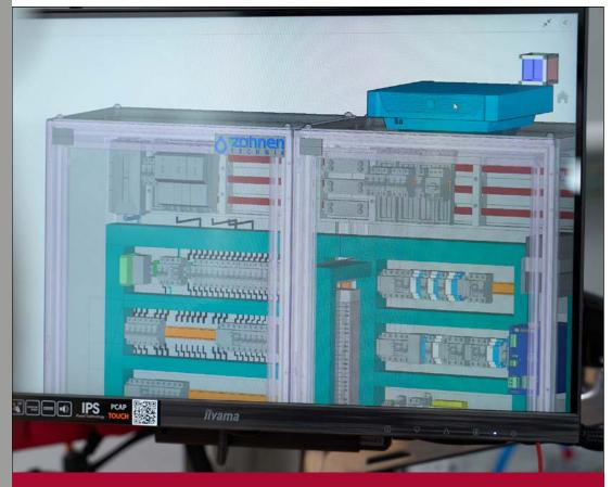
Zahnen works with multi-line and defined connections and has adapted the schematics and 3D macros accordingly to be able to use Eplan Pro Panel for routing.
